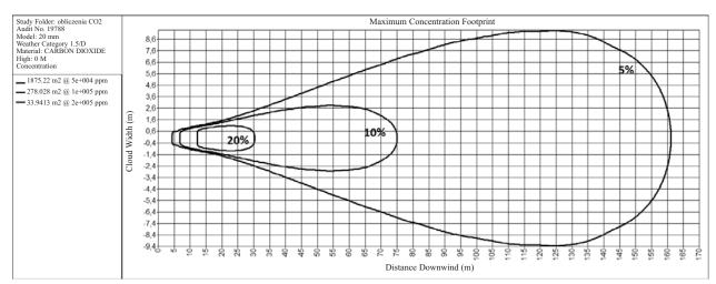
Fig. 6. CO<sub>2</sub> concentration areas for a 0.2 m diameter pipeline.
