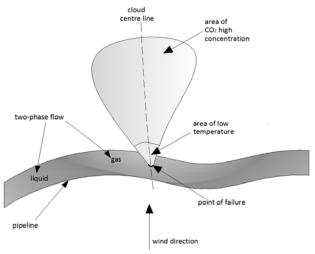
Fig. 3. Gas outflow from the damaged pipeline.
