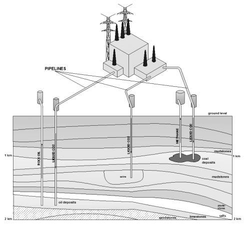
Fig. 1. Possibilities of underground CO<sub>2</sub> storage.
