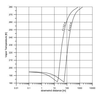
Fig. 4. Change in  $CO_2$  temperature depending on distance from the outflow.
